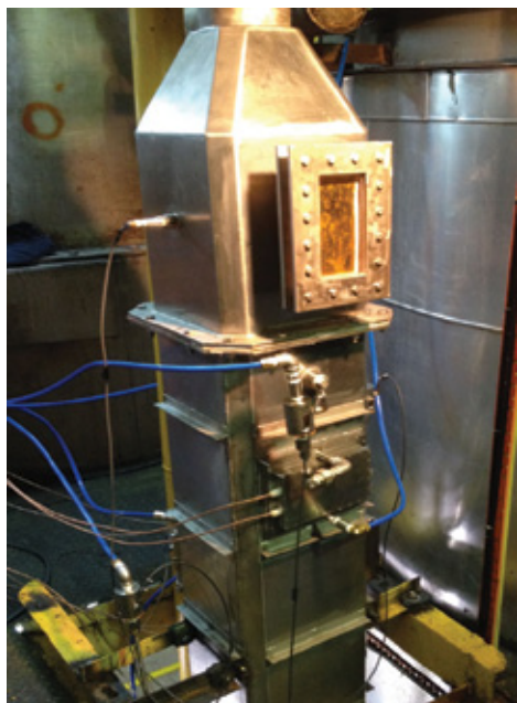
Commercial-scale megasonics reaction chamber in place at the Tai Tak mill.
